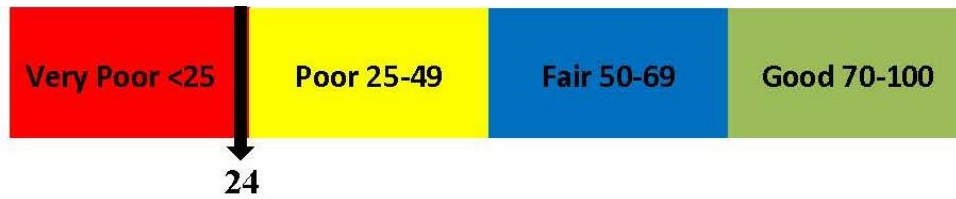
Figure 1. Pavement Condition Categories
